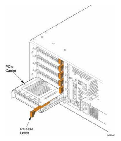
Figure 2-7 PCIe Card Carrier
